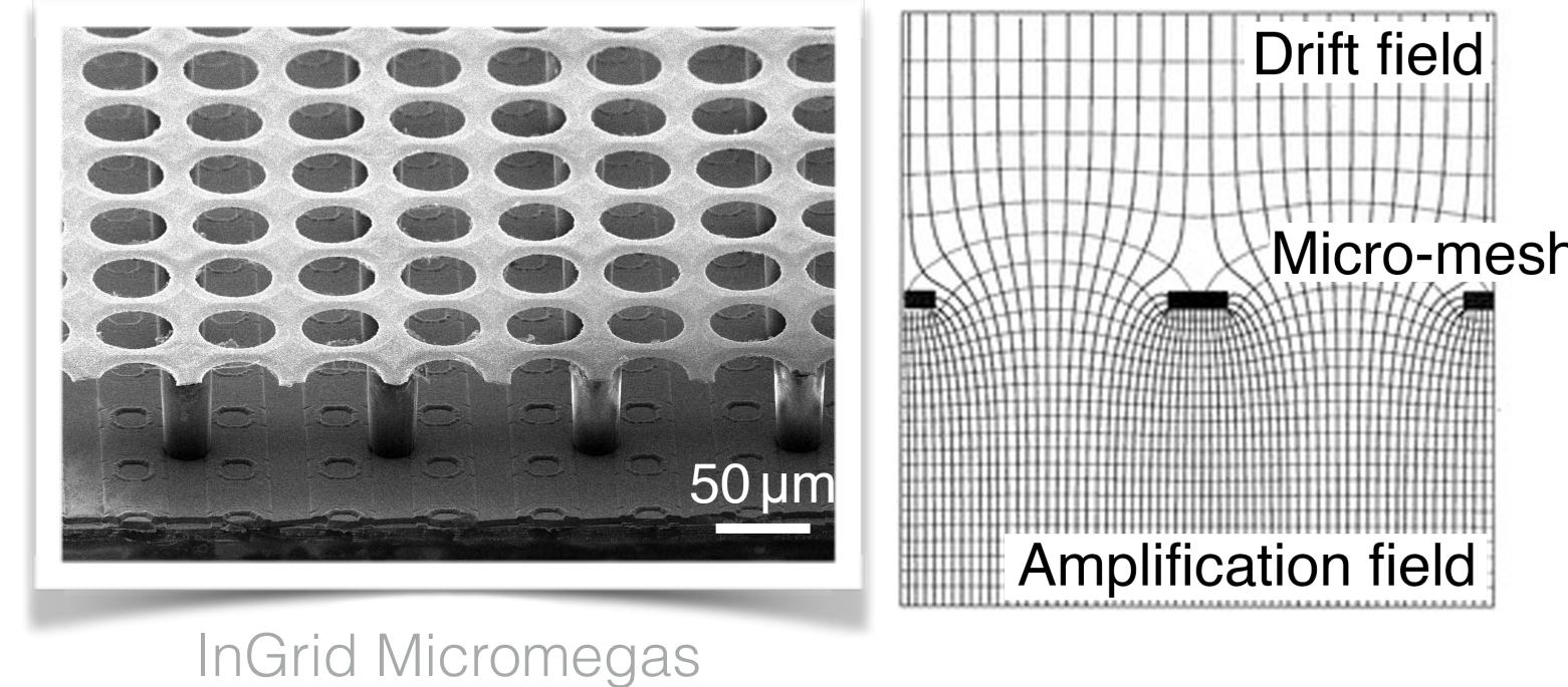
Micro-mesh suspended by pillars above anode.
