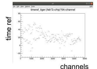
Time reference measurements are affected by time-walk effects and they are biased by low charge hits.
