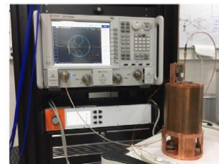
Fig. 8. (a) Drawing of half piece of split cavity. The partition in the middle divides the cavity into two cells when it is assembled. (b) Photo of the system setup consisting of a copper cavity, two rotators under the cavity, a single antenna above the cavity, an actuator controller and a network analyzer.
