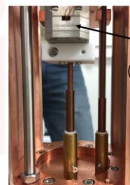
Fig. 8. (a) Drawing of half piece of split cavity. The partition in the middle divides the cavity into two cells when it is assembled. (b) Photo of the system setup consisting of a copper cavity, two rotators under the cavity, a single antenna above the cavity, an actuator controller and a network analyzer.
