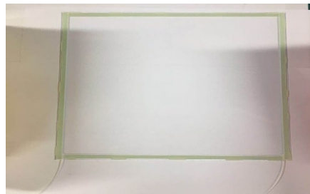
2. Glue walls and pipes.
