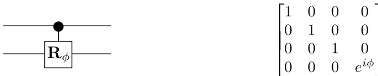
$$|00\rangle \rightarrow |00\rangle \quad |01\rangle \rightarrow |01\rangle \quad |10\rangle \rightarrow |10\rangle \quad |11\rangle \rightarrow e^{i\phi} |11\rangle$$
