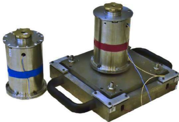
- LAPP active foot + LAPP sensors (one on ground used to monitor ground motion and 1 on top used in feedback) -
