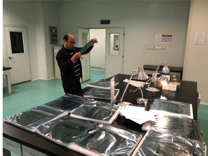
The scintillator strips were wrapped and assembled on EBU boards by Shanghai Institute of Ceramic
