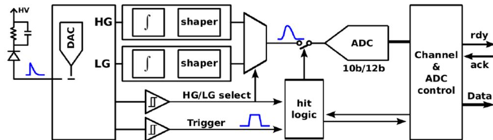
Figure 3.1: Block diagram of the KLauS channel in auto-triggered and auto gain-selection mode.
