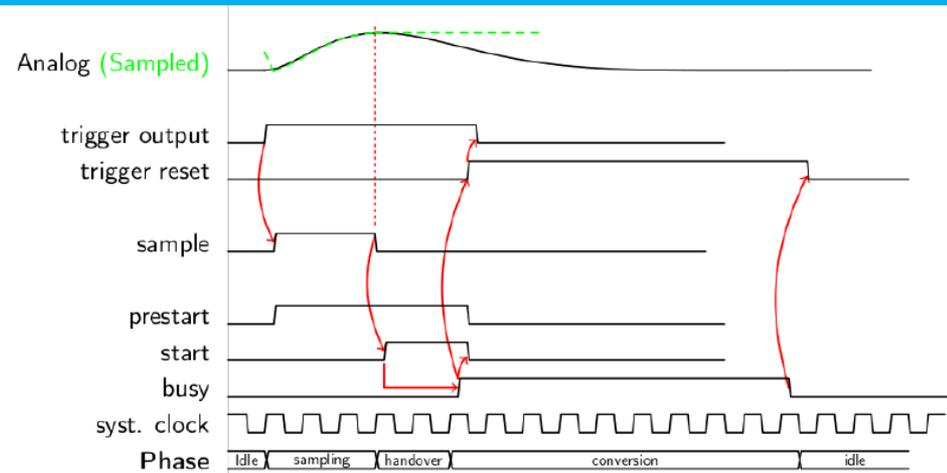
Figure 3.2: Timing diagram illustrating the analog-digital handshake between the hit-logic and the channel control logic.
