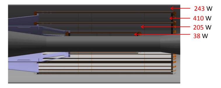
At 200 mW/cm<sup>2</sup> dissipation, the total heat generation is about 900 W, for CEPC level it is about 225 W.
