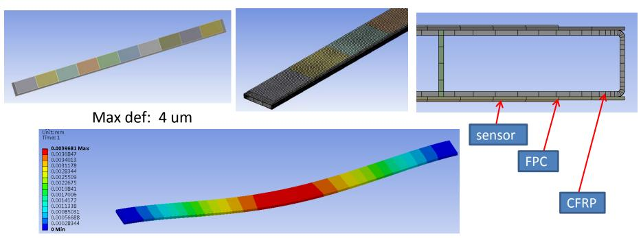
After the FPC with sensors glued on, the rigidity of the full ladder is increased by 24% compare to that of the support itself.
