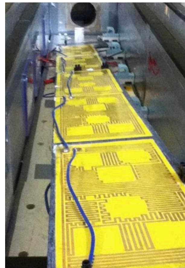
PCB heater for ATLAS strip dummy module
