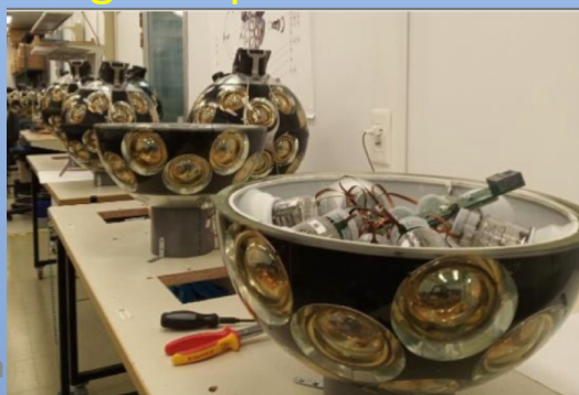
Digital Optical Modules
