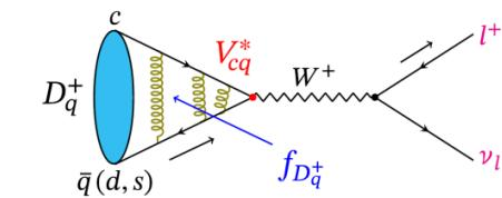
$$\Gamma(D_{(s)}^+ \rightarrow l^+ \nu) = \frac{G_F^2 f_{D_{(s)}^+}^2}{8\pi} |V_{cd(s)}|^2 m_l^2 m_{D_{(s)}^+} \left(1 - \frac{m_l^2}{m_{D_{(s)}^+}^2}\right)^2$$
