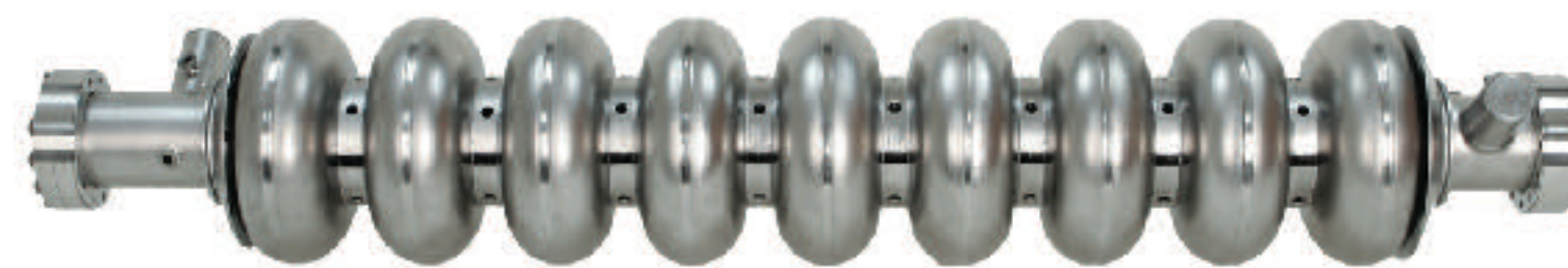
Superconducting RF cavity, average gradient 31.5 MV/m
