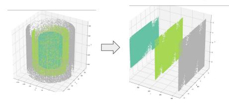
setup tracknet coords as following: phi -> x, z -> y, r -> z
