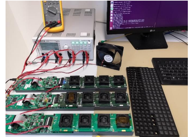
QA test running : 10 ASICs/run , ~100ASICs/hour
