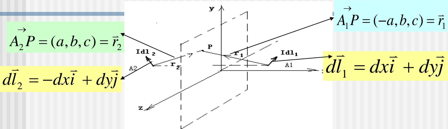
$$d\vec{B}_P \propto d\vec{l}_1 \times \vec{r}_1 + d\vec{l}_2 \times \vec{r}_2$$
