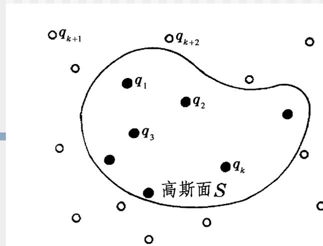
$$\begin{aligned}\Phi_E &= \oiint_S \vec{E} \cdot d\vec{S} = \oiint_S \vec{E}_1 \cdot d\vec{S} + \cdots + \oiint_S \vec{E}_k \cdot d\vec{S} \\ &+ \underbrace{\oiint_S \vec{E}_{k+1} \cdot d\vec{S} + \cdots + \oiint_S \vec{E}_n \cdot d\vec{S}}_{=0} = \frac{1}{\epsilon_0} \sum_{S \text{ 内}} q_i\end{aligned}$$
