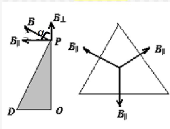
$$B_P = 3 \frac{\mu_0 I}{2\sqrt{3}\pi a} \frac{1}{3} = \frac{\mu_0 I}{2\sqrt{3}\pi a} = \frac{\sqrt{3}\mu_0 I}{6\pi a} \quad \text{方向向上}$$
