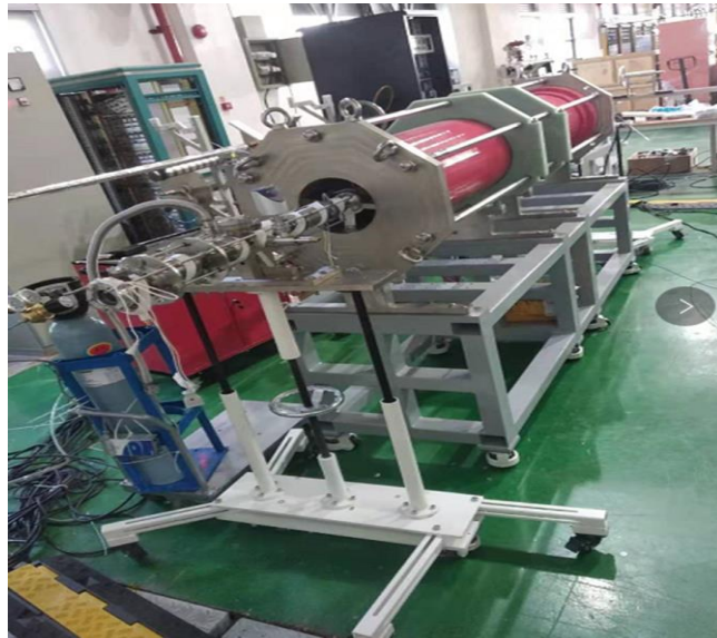
NEG coating setup
