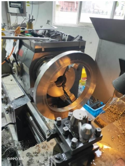
Large flange of UHV tank machining
