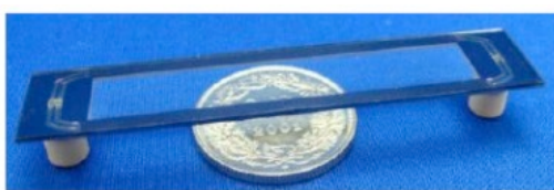
Liquid cooling (mono-phase \text{C}_6\text{F}_{14} @ -20^\circ\text{C} )
