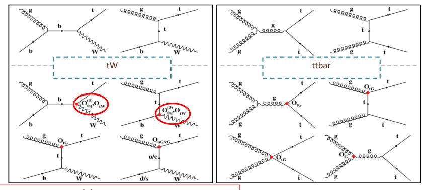
The operators  $O_{\phi q}^{(3)}$  and  $O_{tW}$  modify the SM interaction between W boson, top and b quark (Wtb), its effect can be probed in both top quark decays and single top quark production.
