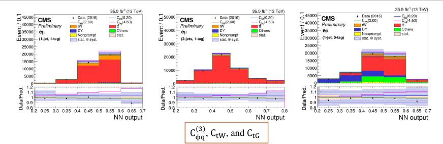
The NN output distributions for data and MC in different categories used in the limit setting.
