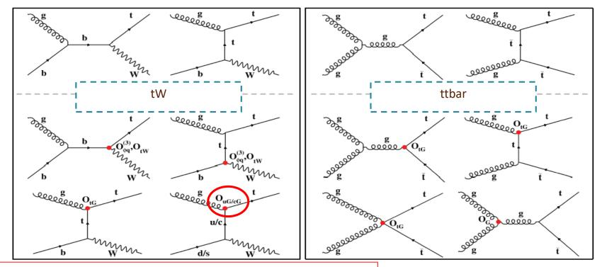
The operators  $O_{cG}$  and  $O_{uG}$  lead to flavor changing neutral current (FCNC) interactions of top quark and contribute to the tW production.
