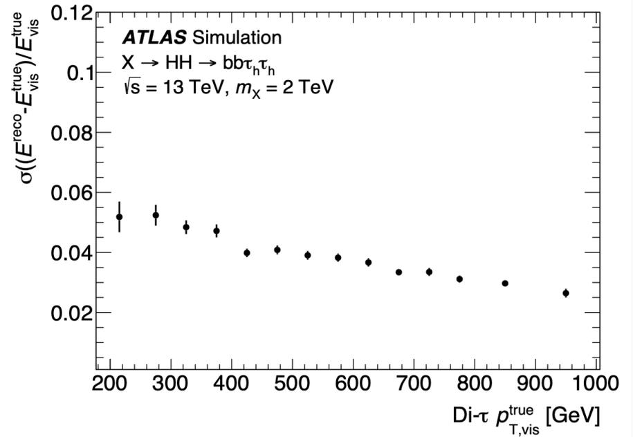
Energy scale and resolution of the di- $\tau$  reconstruction as a function of the  $p_T$  of the di- $\tau$  system at generator level.
