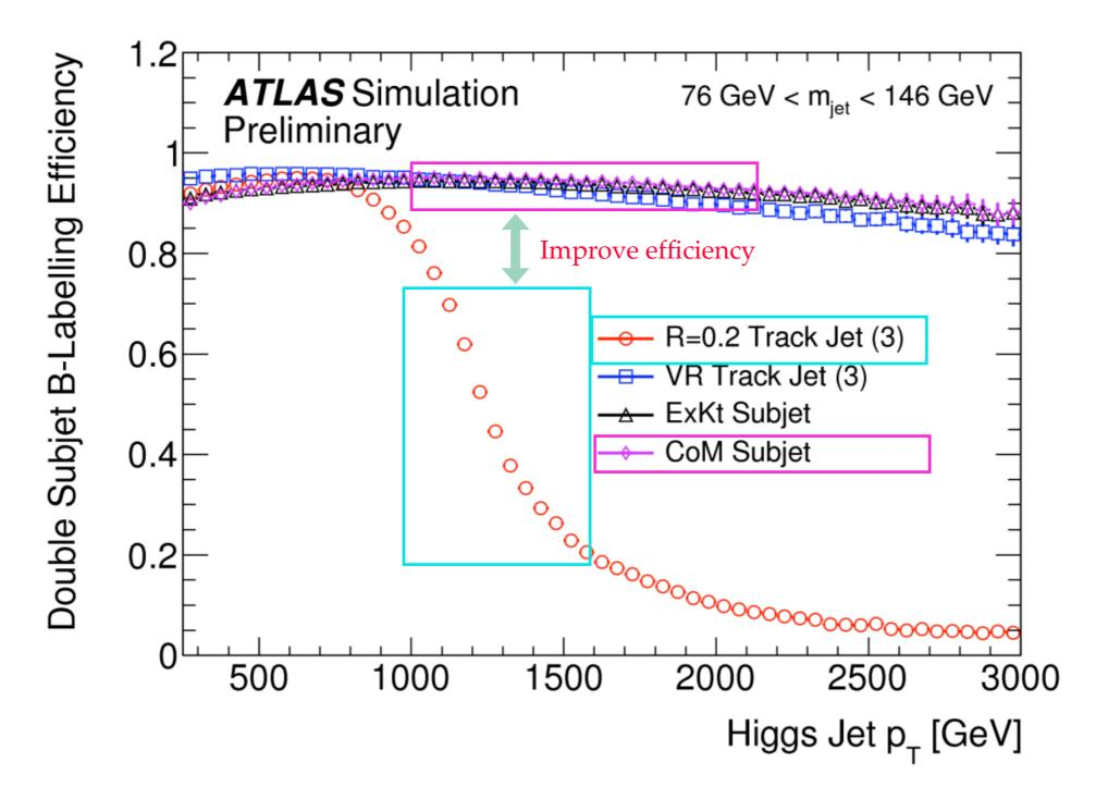
The efficiency of CoM jet is much better than the R=0.2 track jet for high Jet pT (pT>1000GeV)
