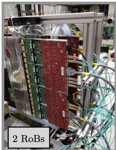
2 final Modules+FEE tested successfully with 450 GeV protons @CERN in July 2018
