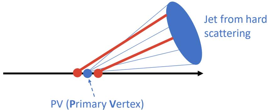
$$R_{p_T} = \frac{\sum p_T^{\text{trk}}(\text{PV}_0)}{p_T^{\text{jet}}} \begin{cases} R_{p_T} > s, & \text{Hard scattering jet} \\ R_{p_T} < s, & \text{Pile-up jet} \end{cases}$$
