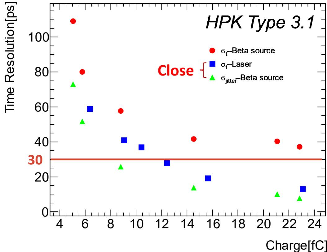
$$\sigma_t^2 = \sigma_{\text{Landau}}^2 + \sigma_{\text{timewalk}}^2 + \sigma_{\text{jitter}}^2$$
