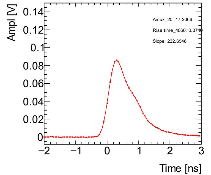
$$\sigma_{\text{jitter}} = \frac{\text{RMS}}{\text{slope}} = \frac{\text{RMS}}{\frac{\text{Ampl} * 20\%}{T_{60\%} - T_{40\%}}}$$
