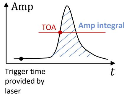
$$t_{\text{TOF}} = t_{\text{TOA}} - t_{\text{trigger}}$$
