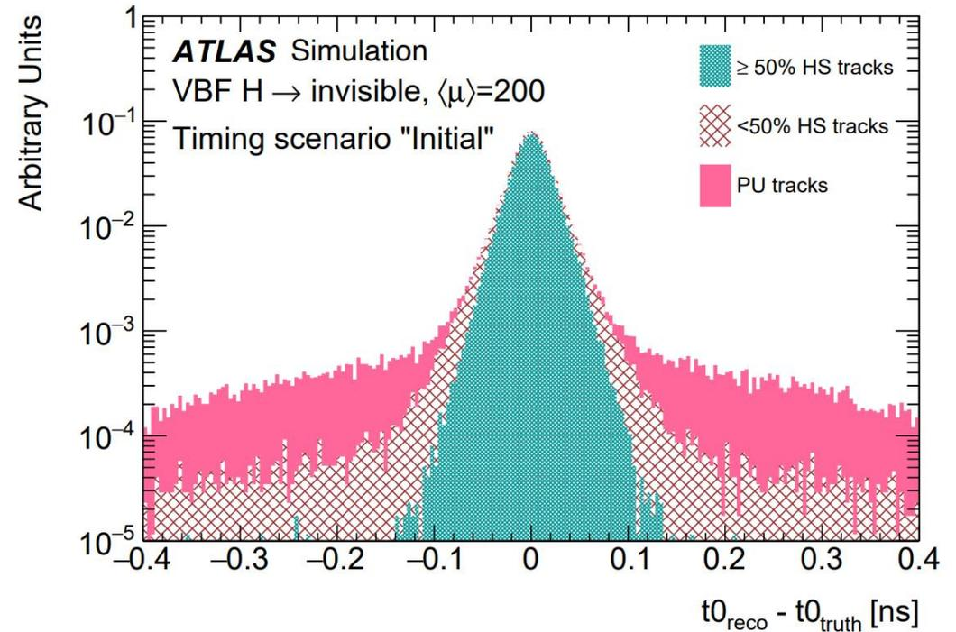
$t_{\text{reco}}^0 - t_{\text{truth}}^0$  distribution for VBF H(inv) events
