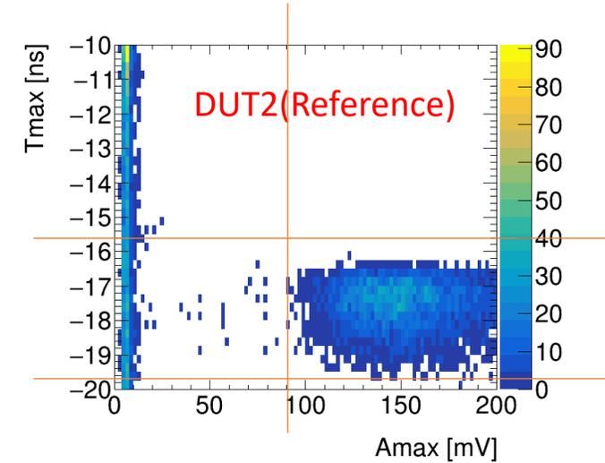
*Tmax: time when the amplitude of the waveform gets maximum*
