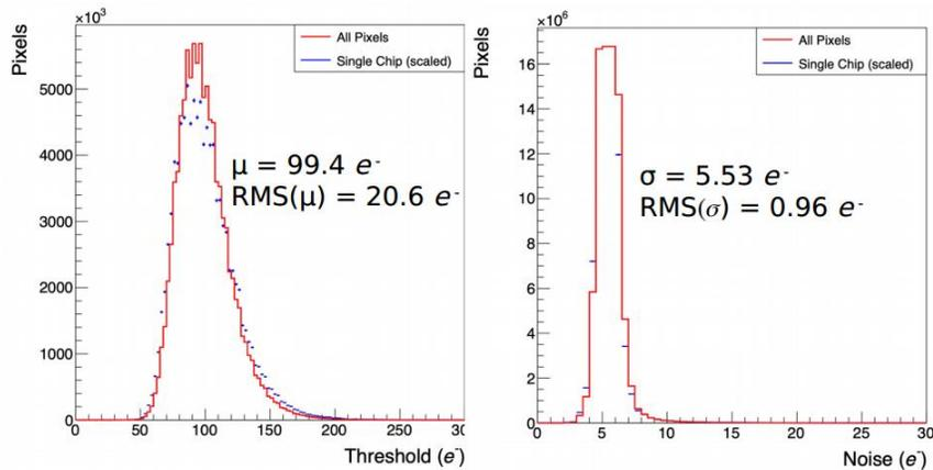
Threshold and noise after tuning an OL stave (~100 M pixels) compared to test data from a single chip
