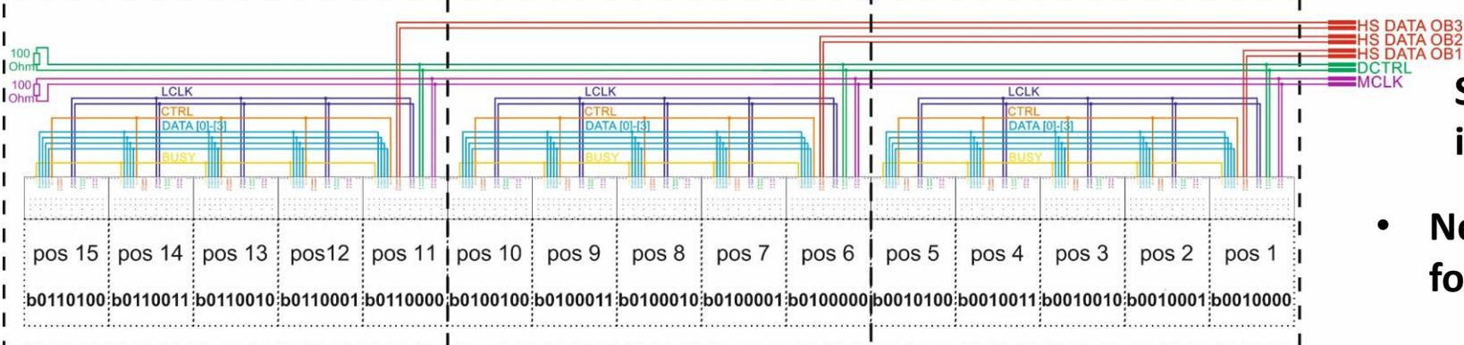
Schematic diagram of the electrical interconnections for OBs only
