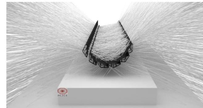
Cosmic tracks in one half layer of the Inner Barrel
