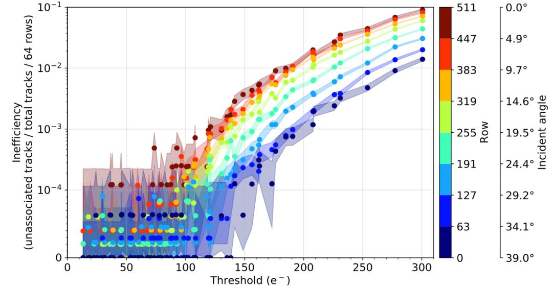
Fig. 10: Inefficiency as a function of threshold for different rows and incident angles with partially logarithmic scale ( $10^{-1}$  to  $10^{-5}$ ) to show fully efficient rows. Each data point corresponds to at least 8k tracks.
