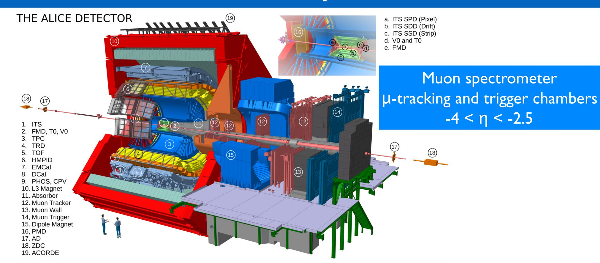
Central barrel: vertexing, tracking, PID, EM Calos  $|\eta| < 0.9$
