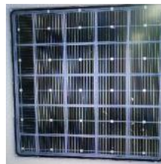
IHEP-NDL LGAD-V2 Pixel size 1.3 \times 1.3 \text{ mm}^2
