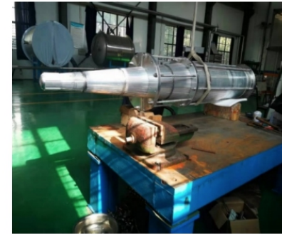
150kW beam collector
