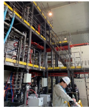
Large size baking furnace commissioning
