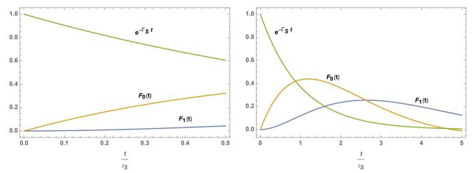
Shown are  $F_0(t)$ ,  $F_1(t)$ , and  $\exp[-\Gamma_S t]$ , plotted over a short time interval of relevance to LHCb (left), and a longer time interval of relevance to Belle-II (right)
