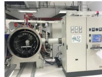
Vacuum furnace (doping & annealing)
