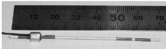
FIGURE 2. The aluminum sample cut from the aluminum stabilized superconductor attached with a voltage sense wire.
