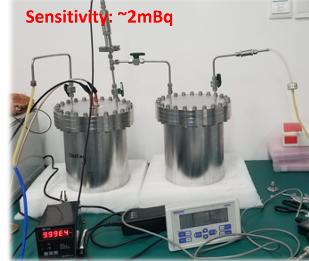
Radon emanation measurement system(SJTU)
