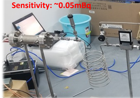
Cold trap radon emanation system(SJTU)
