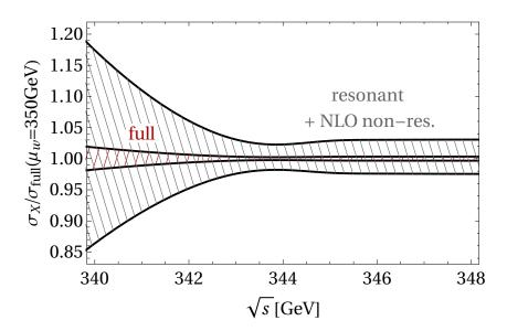
Figure 13: The resonant plus NLO non-resonant (grey hatched band) and full cross section (red hatched band) are shown for  $\mu_r = 80 \,\text{GeV}$ . The bands are the envelope of the values obtained by varying  $\mu_w$  between 20 and 700 GeV. The results have been normalized to the full cross section for the central scale  $\mu_w = 350 \,\text{GeV}$ .
