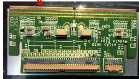
Full Module Hybrid+Flex PCB
