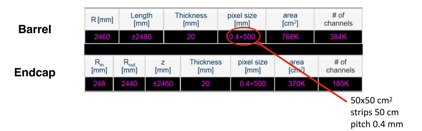
IDEA's Preshower detector would have in total: Barrel 77x2 m<sup>2</sup> (154 m<sup>2</sup> total) Barrel 384000x2 channels Endcaps 37x2 m<sup>2</sup> (74 m<sup>2</sup> total) Endcaps 185000x2 channels
