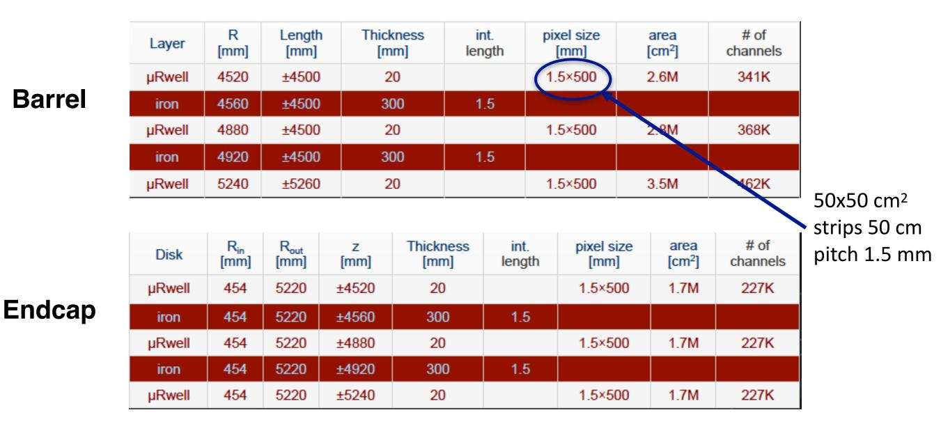
IDEA's Muon detector would have in total: Barrel 900x2 m<sup>2</sup> (1800 m<sup>2</sup> total) Barrel 120000x2 channels Endcaps 500x2 m<sup>2</sup> (1000 m<sup>2</sup> total) Endcaps 680000x2 channels
