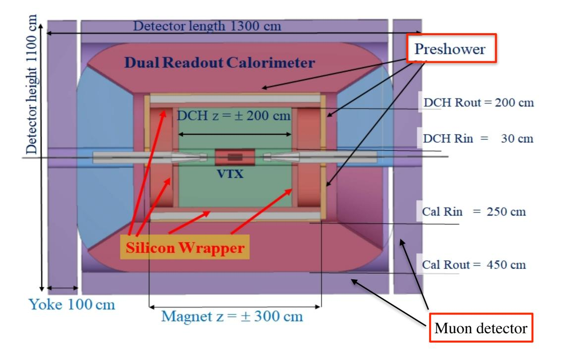
Preshower and the muon detection system are designed with the µRWELL technology
