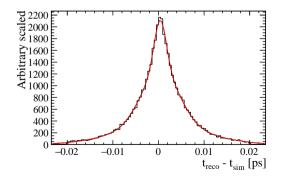
Obtained from detector simulation. Proper decay time:  $t = \frac{m l_{xy}}{p_{\rm T}}$ Fit with sum of three gaussian.
