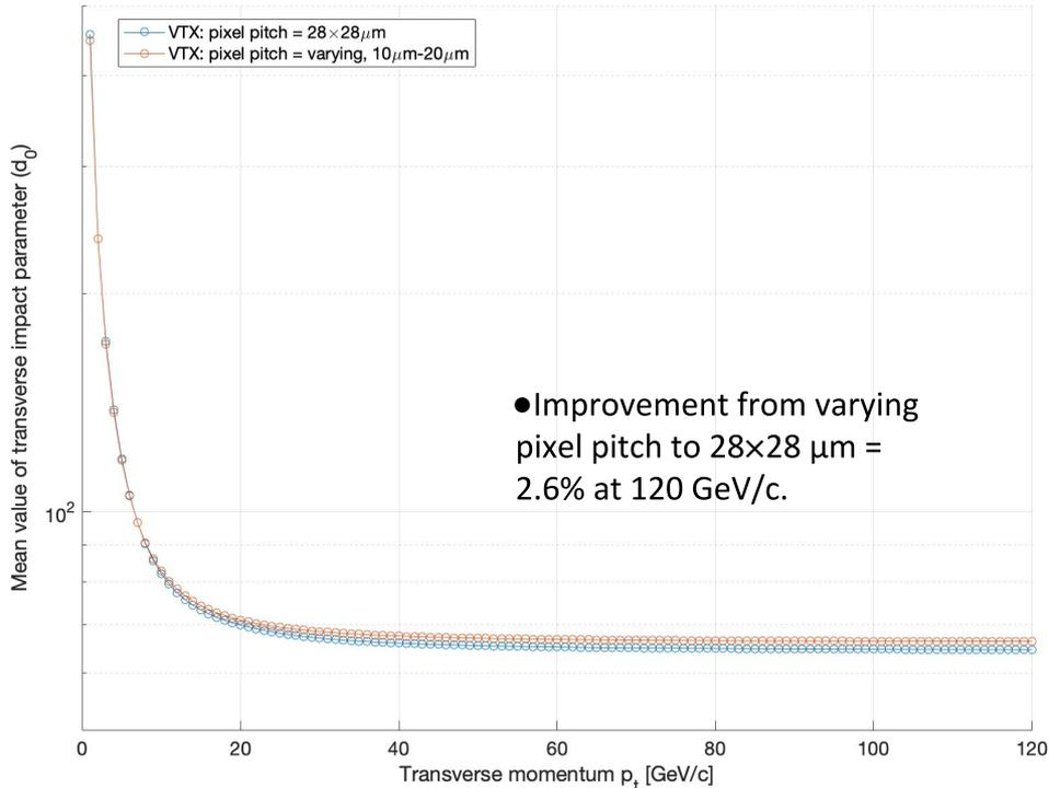
Impact of varying material budget in VTX detector on mean transverse impact parameter ( $d_0$ )
