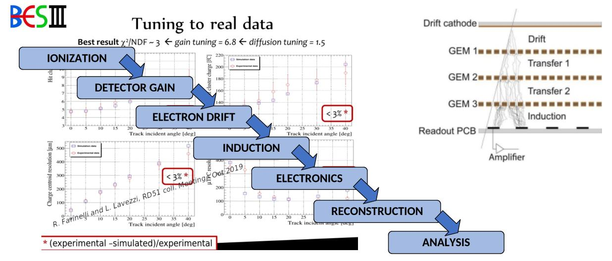
A triple-GEM parametric simulation which take into account diffusion, transparency, gain, induction and readout electronics has been developed within the CGEM-IT BESIII frame. The simulated data has been tuned to the experimental results of charge, multiplicity and spatial resolution (CoG and µTPC)
