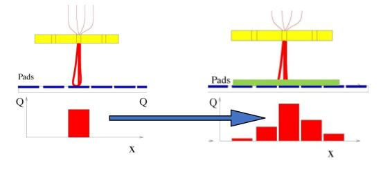
Modified GEM anode with a high resistivity film bonded to a readout plane shows the improvement introduced by the charge dispersion with respect to a design without a resistive film.
