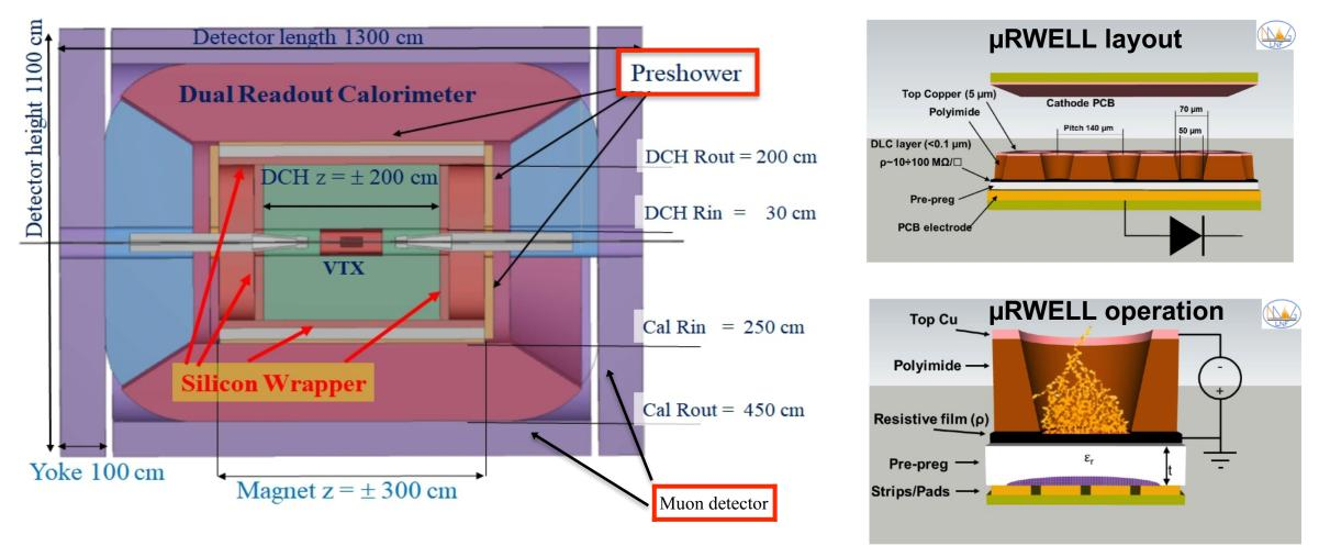
Pre-shower and the Muon Systems are designed with the µRWELL technology
