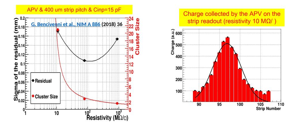
The use of low resistivity increases the charge spread (cluster size) on the readout strips and then  $\sigma$  is worsening. At high resistivity the charge spread is too small (CI\_size  $\rightarrow$  1) then the Charge Centroid method becomes no more effective ( $\sigma \rightarrow \text{pitch}/\sqrt{12}$ ).
