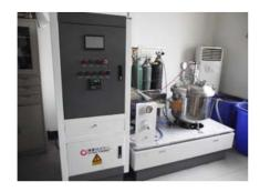
Microwave sintering (MWS) (30min.)
