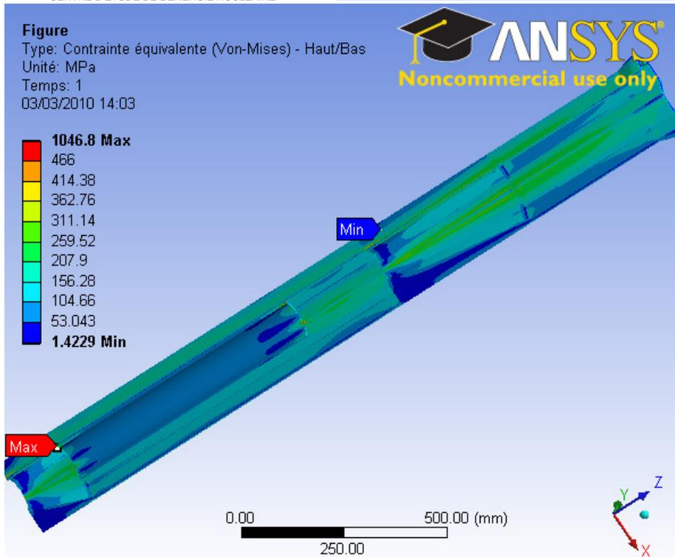
0.5 MP external pressure 100K  $\Delta T$  , 4mm wall thickness
