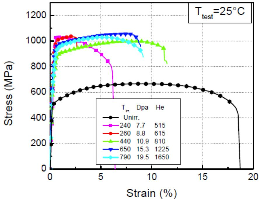
*STIP-III irradiation data of T-91 steel at different irradiation temperatures.
