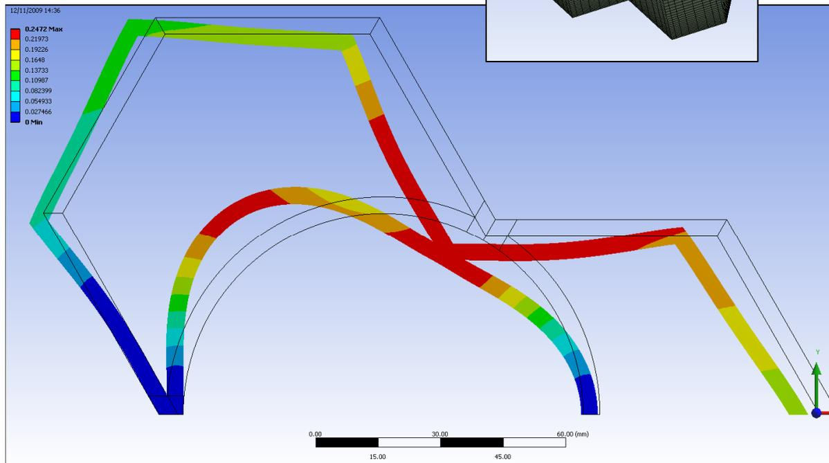
1 MP external pressure, 4mm wall thickness
