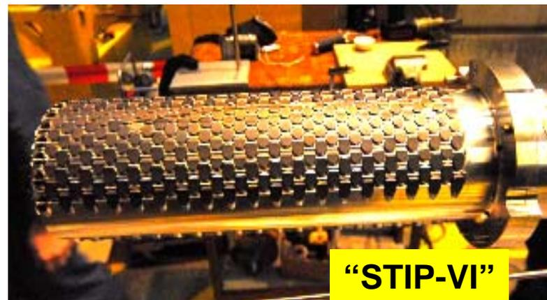
Max. Proton flux:  $2.4 \times 10^{14}$  p/cm<sup>2</sup>/s.
