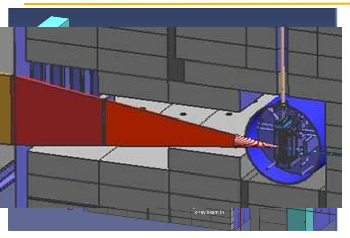
High fluence, high energy, low divergence X-ray sources offer the potential of placing detectors far from the sample
