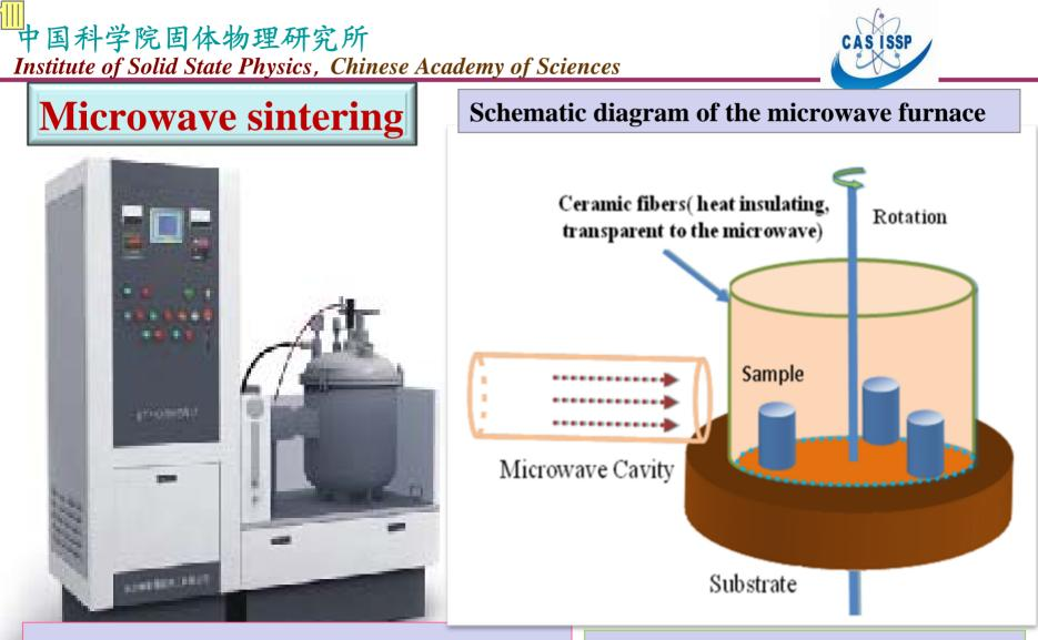
Main parameters of microwave furnace sintering space: Φ150 × 160 (mm) maximum Temperature: 1600 °C Microwave frequency: 2.450GHz reducing atmosphere (5% $H_2$  and 95%Ar).
