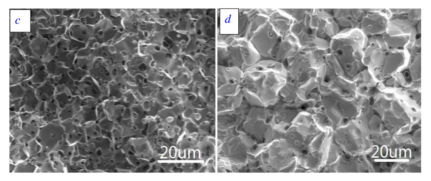
(c) coarse powder sample sinteredat 1400C (30min):
