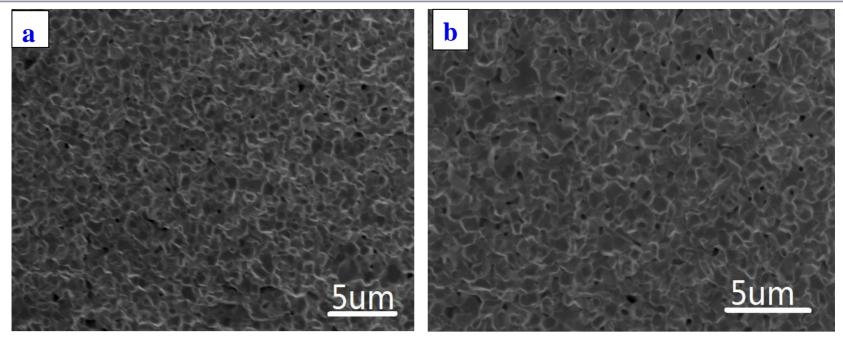
(a) nano powder sample sintered at 1500C (30min): 1 μm; density: 95%
