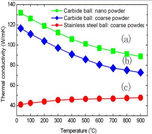
(1) nano powder sample shows the highest thermal conductivity among the three samples (max: ~140 W/mK);
