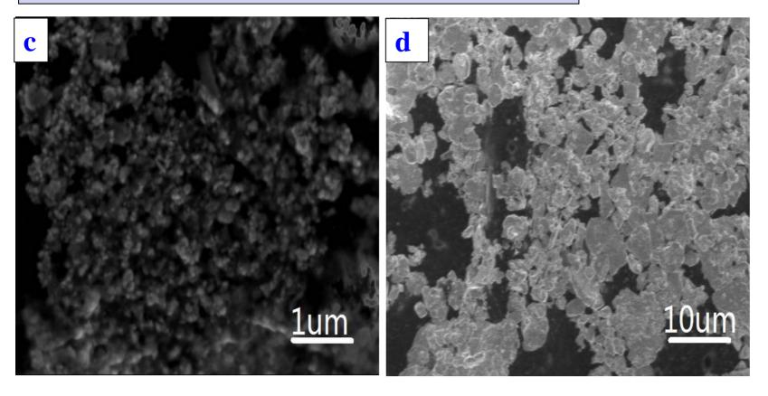
(c) Nano powder: the agglomeration is almost eliminated;(d) Coarse powder: the surface is smoothened
