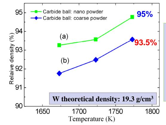
Temperature dependence of sintering density of bulk W
