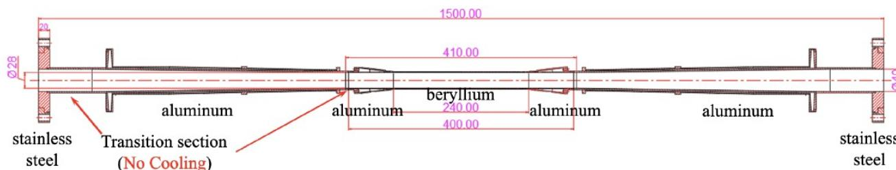
Smaller Be pipe radius preferred to fabricate thinner beampipe (less material)
