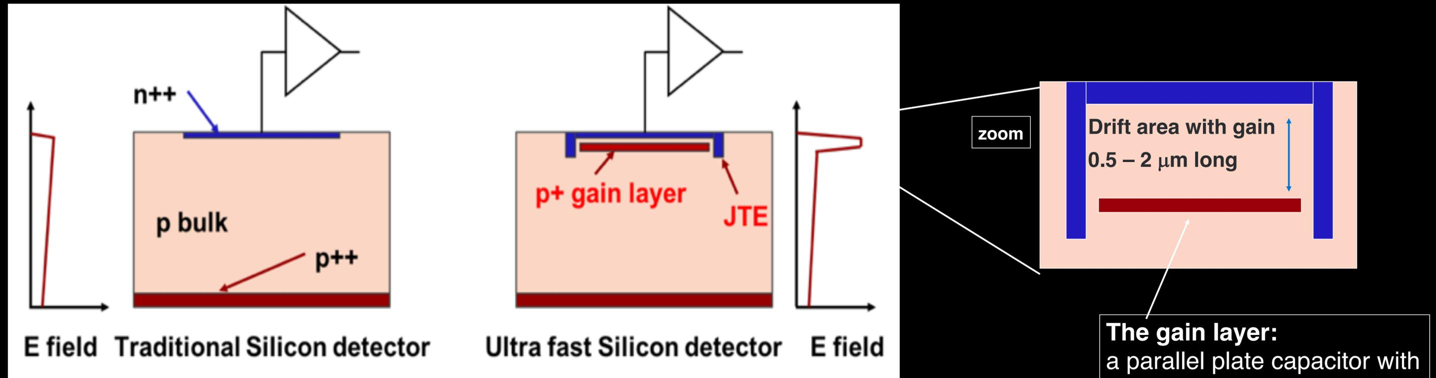
**The LGAD sensors, as proposed and first manufactured by CNM**
