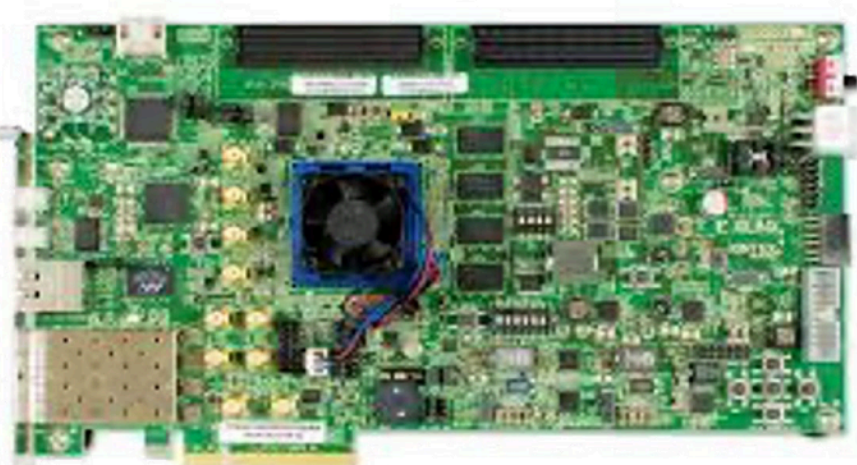
Xilinx Kintex UltraScale FPGA KCU105 Evaluation Kit chosen to be compatible with CAEN digitizer boards
