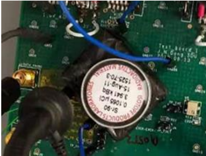
TaichuPix1 response to ^{90}\text{Sr} beta source
