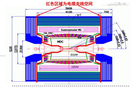
About 20000 cables at the endcap of BESIII detector, which are about tens of meters in length
