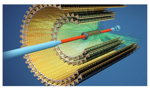
The silicon pixel detector is the first choice for the vertex detector of colliding physics experiments
