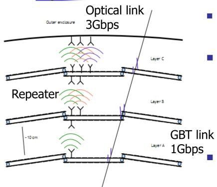
Proposal of a radial readout for the tracker detector of the ATLAS experiment
