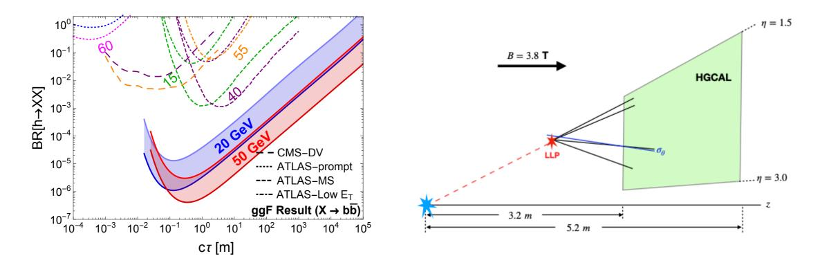
Using the pointing capability of CMS HGCAL Best sensitivity  $\approx 10^{-7}$ , can reach  $c\tau \approx 10^3$  m with BR  $\approx 10^{-3}$ In addition, precise timing could also help.
