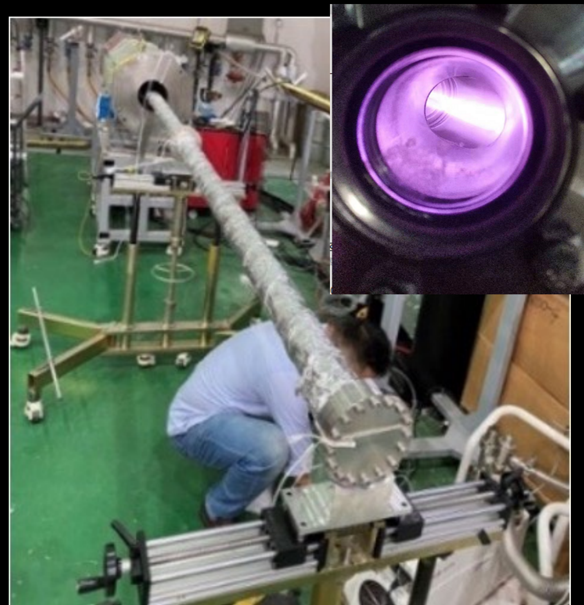
NEG Coating setup (6 m tubes)
