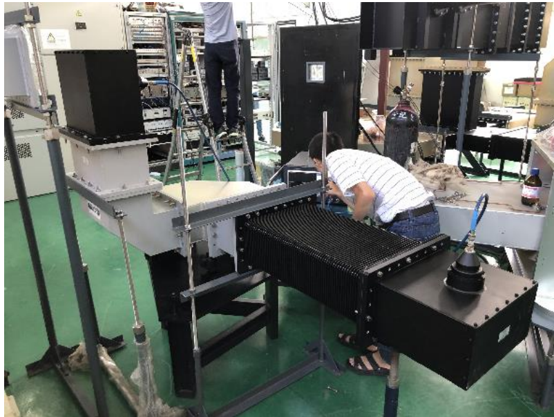
Cold test for waveguide system
